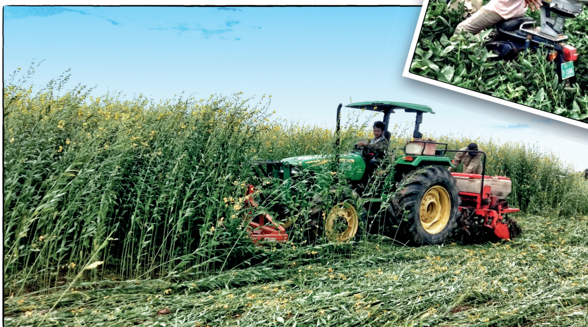
Photo4: Use of roller crimper for planting green of maize on sunnhemp, Rattanak Mondoul, Battambang, June 2018
