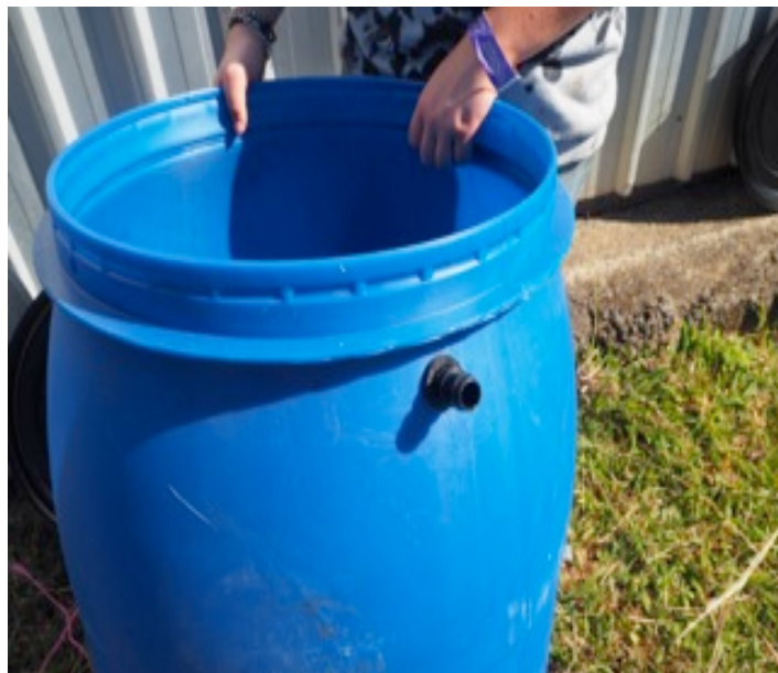
Insert a fitting into the airlock
