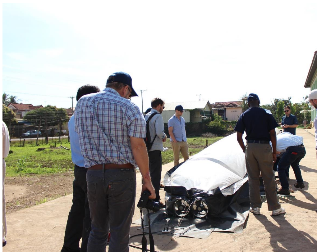
Fig. 4: Solar bubble dryer from Grain Pro, Bos Khnor Station; capacity of 2 tons.
