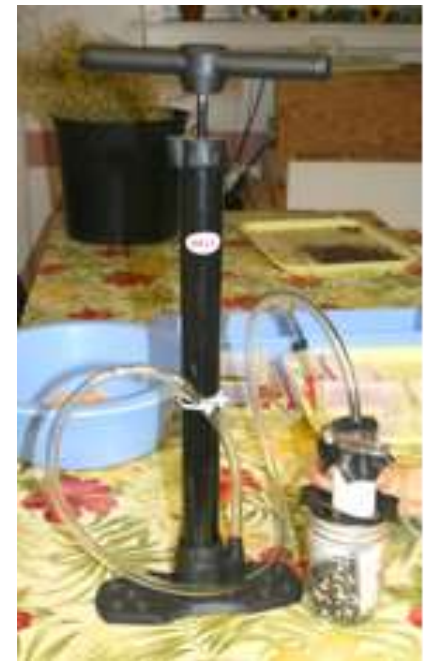
Figure 1. The vacuum packing system for seed storage.
